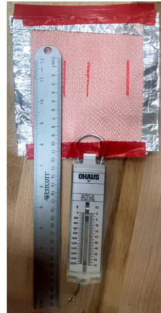
Fig. 4. Characterizing the Stress/Strain Curve of Nextel 440
